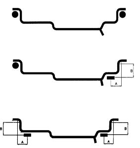
Alu 3: A standard clip-on weight is used on the inner rim flange and a stick-on weight is applied towards the center area of the rim. This is a 'hidden-weight' technique - the weights should not be visible when the wheel is replaced on a car.
